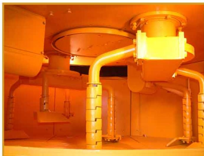
Internal View of Planetary Mixer, 立轴行星式搅拌机内部
